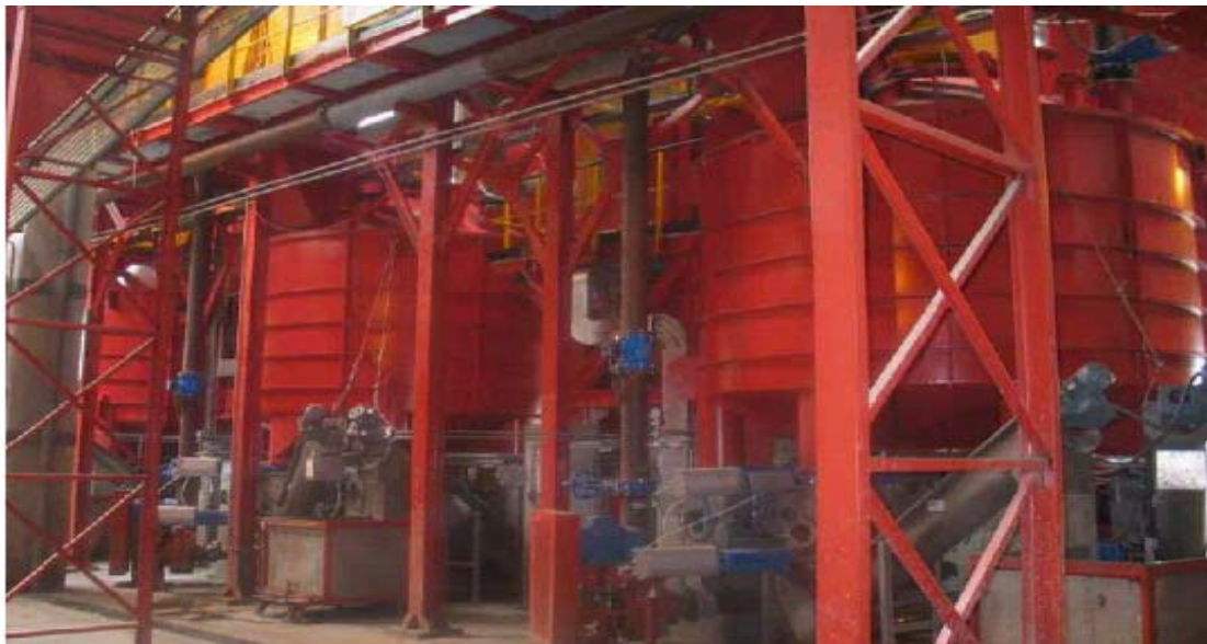
Figure 5 32 m³ BTA pulper in Ca' del Bue, Verona
