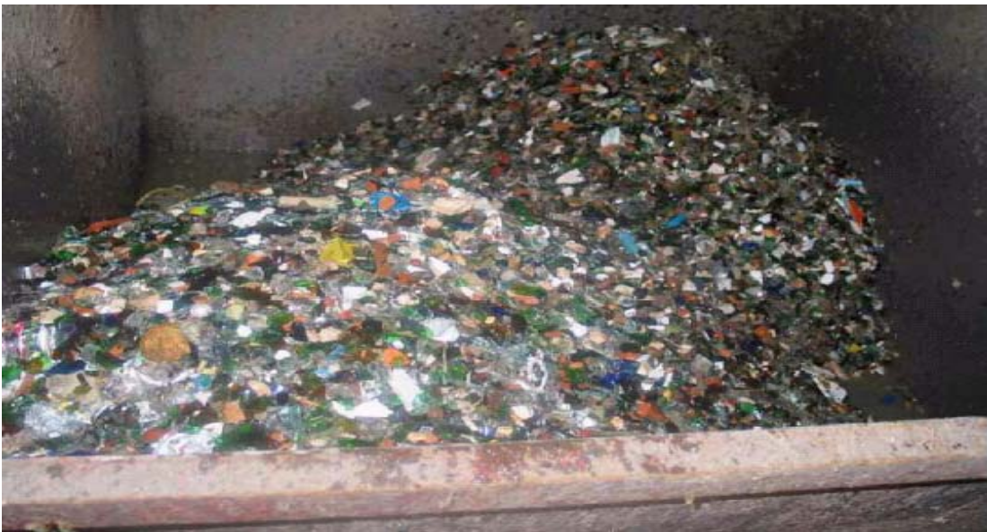
Figure 7 Separated heavy fraction of the wet-mechanical processing
